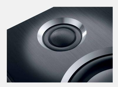
The Edelstein is a gem: a Kapton voice coil mount drives an aluminium oxide-ceramic sandwich cone in the bass range. From 2500 Hz the pulses are transferred to a silk dome that Magnat has elegantly installed behind a conically machined front panel, which functions effectively as a sound guide.
